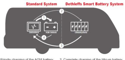
1. Priority charging of the AGM battery 3. Discharging the lithium battery Complete charging of the lithium battery
